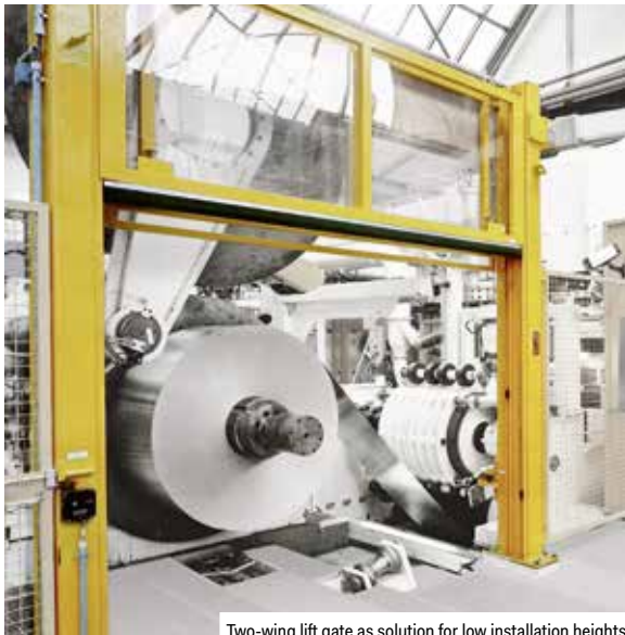
Two-wing lift gate as solution for low installation heights
