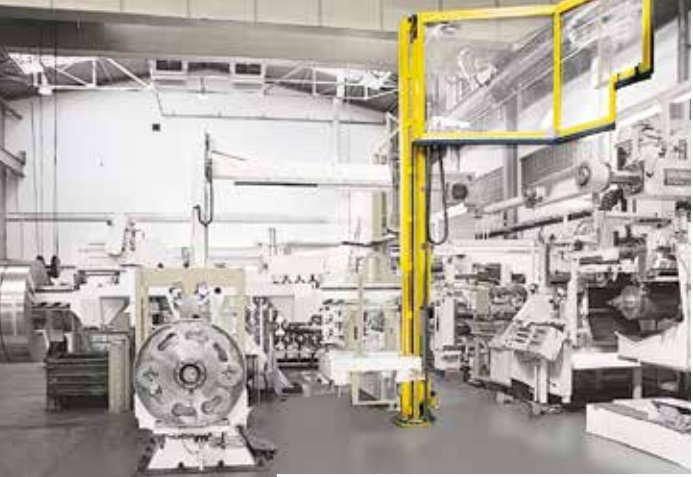
Single-sided lift gate with offset wing shape + contour cut-out
