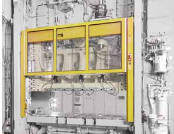
Compact machine protection gate as process integration with low installation height
