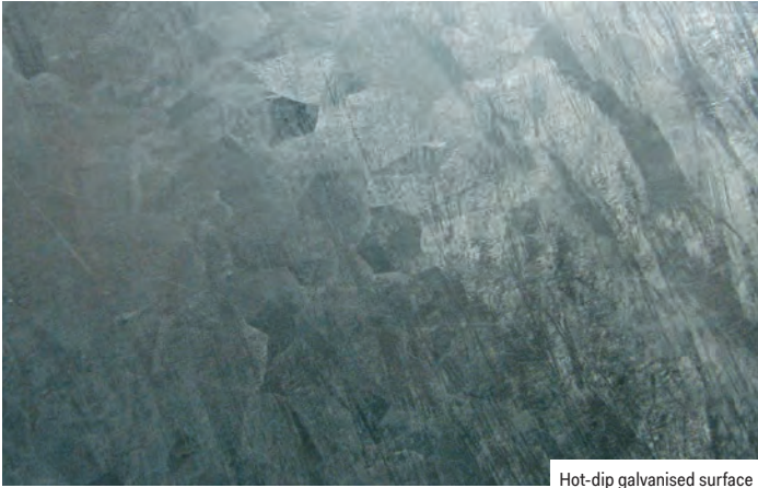
Hot-dip galvanised surface
